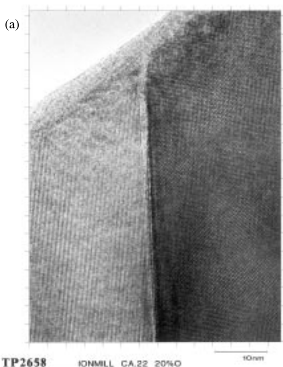
Fig. 1. TEM image (a), and elemental distribution in the vicinity of a grain boundary of \text{La}_{0.80}\text{Ca}_{0.22}\text{CrO}_3 (b) and \text{La}_{0.70}\text{Ca}_{0.32}\text{CrO}_3 (c).
